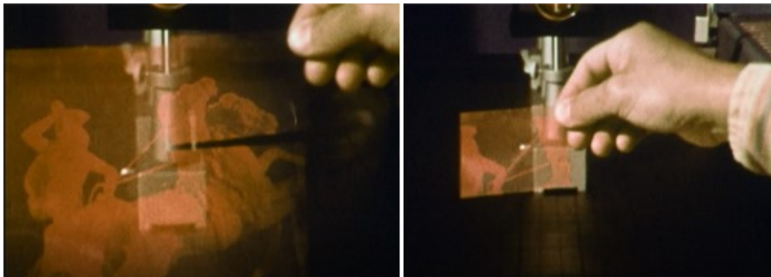
Figure 1: Every piece of the holographic film can reconstruct the entire image, stills from the video [4]
